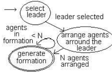
Fig. 2. General algorithm to generate static formations for N agents
